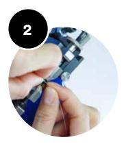
**ATTACHING PROCESS** Surgical sutures attaching machine provides a secure way to attach drilled end
